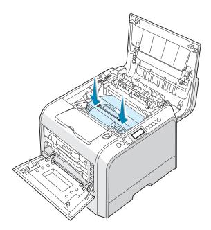
**14** Firmly push the lock levers on each side towards the top cover, as shown below, to lock the transfer belt into place.
